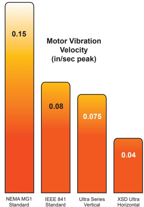
**It is well documented that motors designed with low vibration have longer bearing life.**
